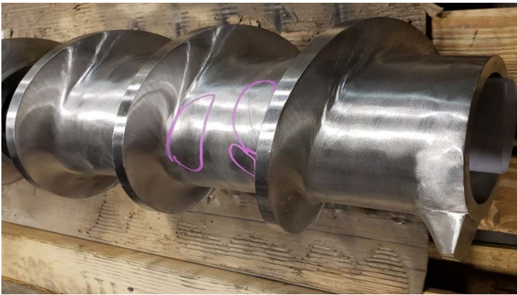
Figure 3- Visible cracks on near finished casting
