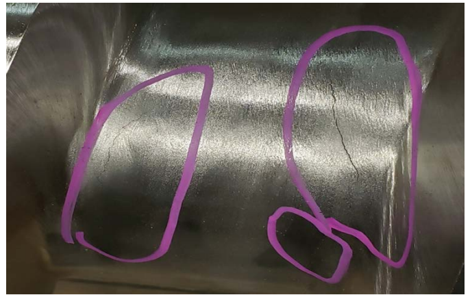
Figure 4- Visible cracks on near finished casting
