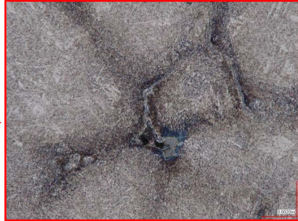
Figure 29- Location 1, Sample A, adjacent to riser. Vilella's Reagent. Magnification: X800
