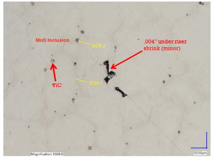
Figure 15- Location 1, magnification: X500
