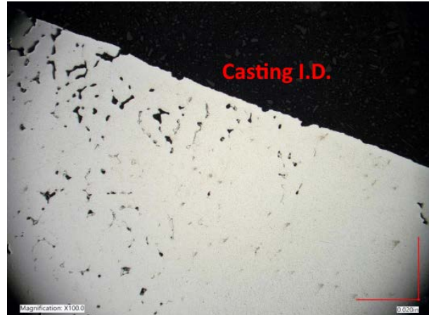
Figure 27- Location 2, opposite of riser. Unetched
