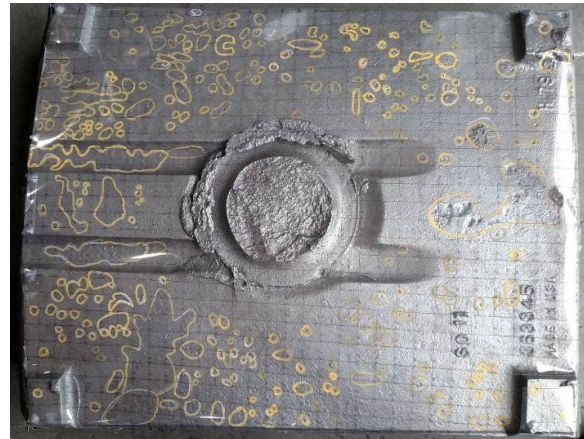
Inclusions Marked for Repair on Casting Cope Surface
