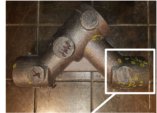
Inclusions Marked for Repair
