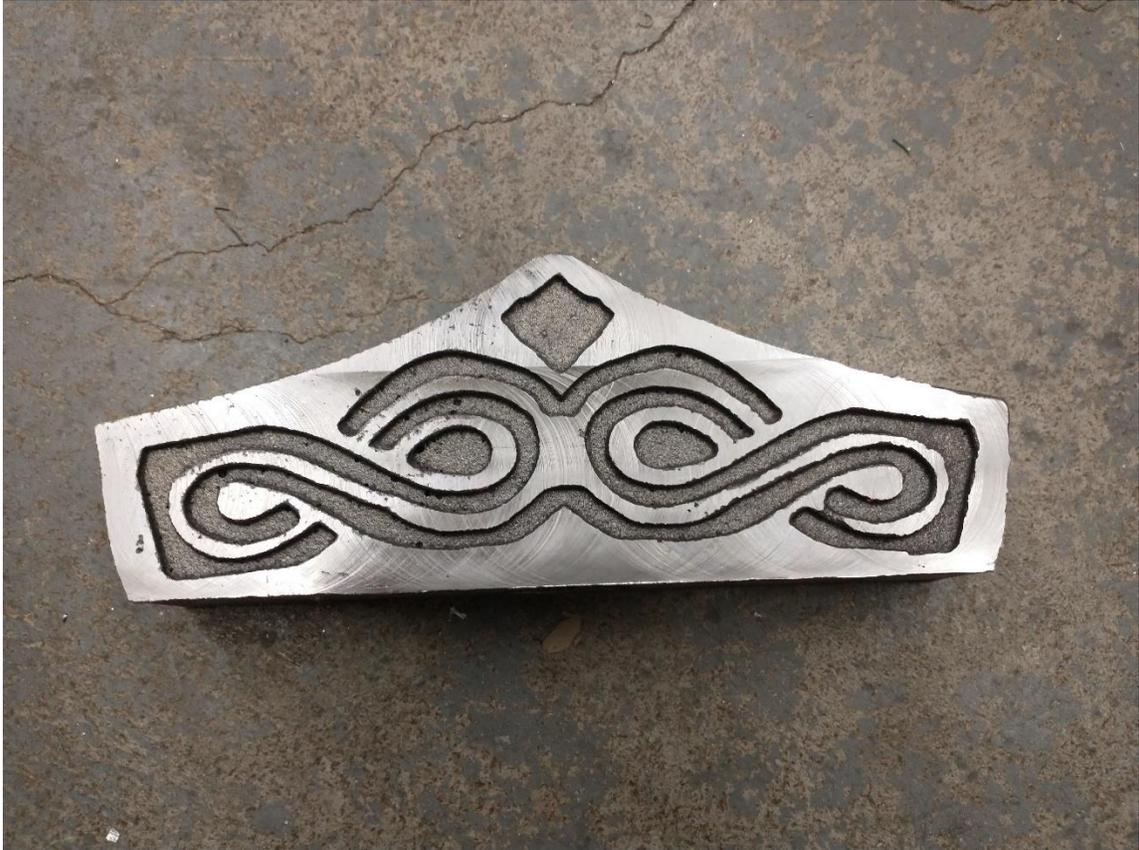
Following machining, the hammer went through heat treating to increase its hardness. To heat treat, we held the hammer head in a furnace for 2 hours at 700° C, followed by quenching in oil. After the hammer was cool enough to remove from the oil, it was left to air cool. Heat treating and quenching also gave the hammer a dark appearance and highlighted the runic design more, finishing the appearance of the head itself.
