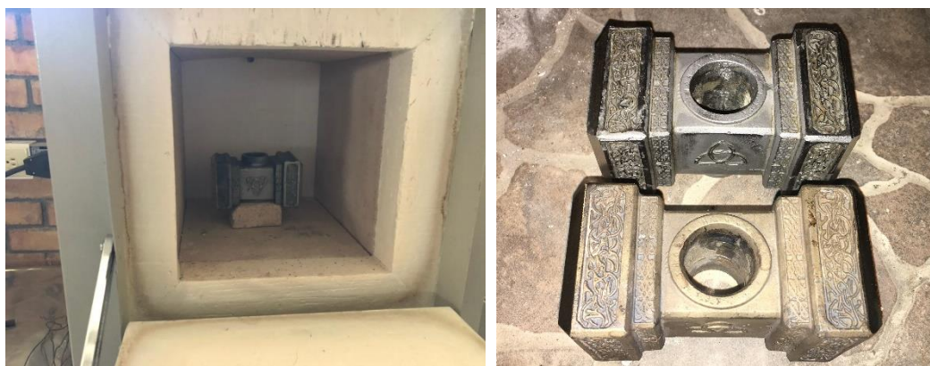
Figure 4.7. Heat treated hammer showed a characteristic gold color after treating.
