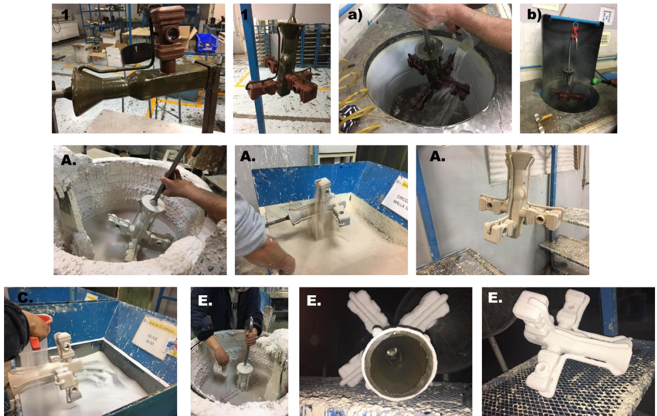
Figure 4.4. Investment process. Letters and numbers indicate the respective step.
