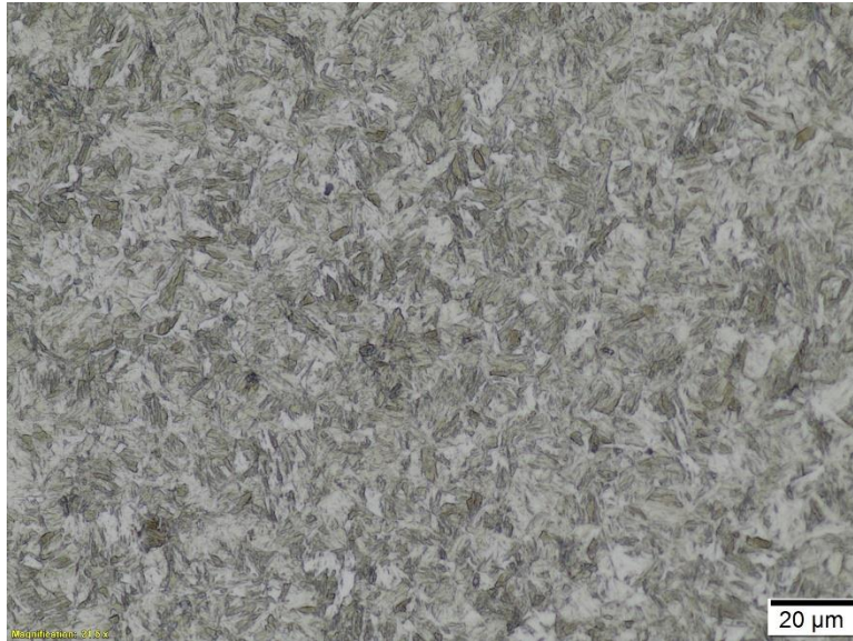
Figure 40: High Magnification Image of Quenched 8630 Steel Microstructure
