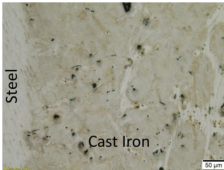
Figure 35: Medium Magnification Image of Bimetal Interface As-Cast
