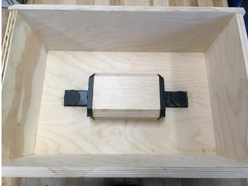
Figure 27: Matchplate Pattern for Flaskless Chemically Bonded Sand Mold
