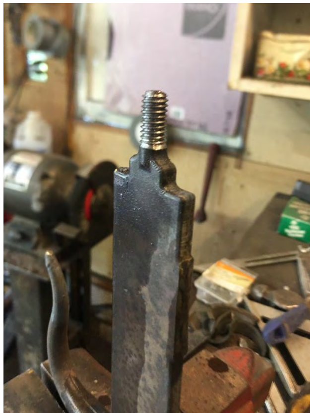
5/16 – 18 Thread on End of Casting
