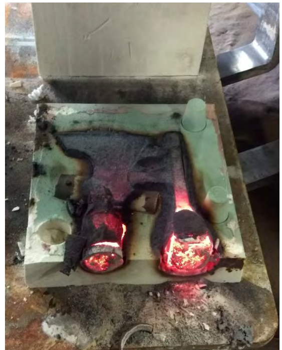
Figure 5- The axe cooling in half of the mold.
