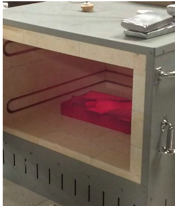
Figure 9 - Normalization of the axe.
