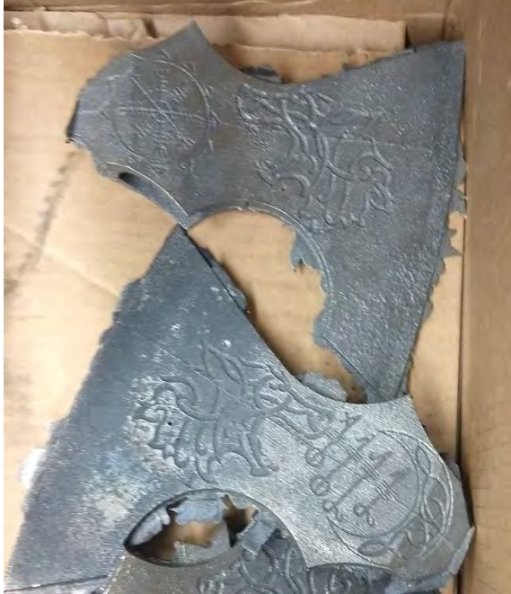
Figure 6 - Axe heads after the gating was removed.
