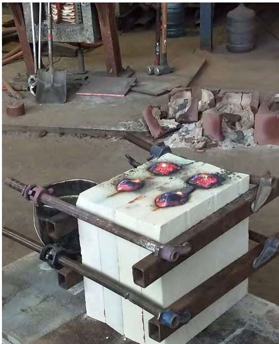
Figure 4 - Steel cooling inside of the mold.
