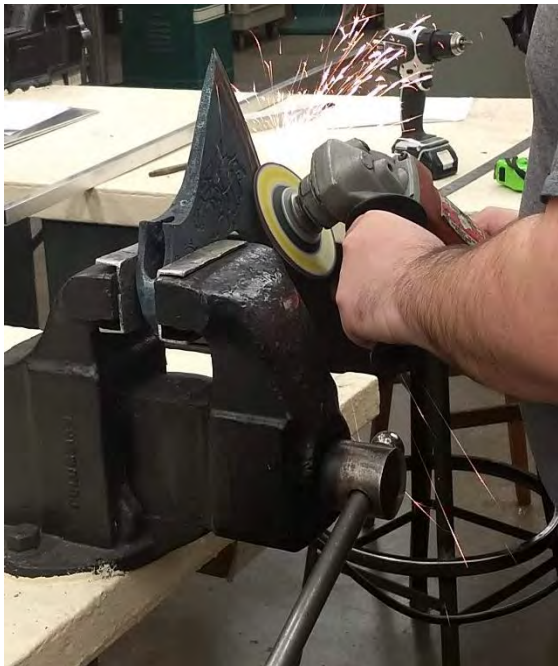
Figure 8 - Grinding to adjust the blade's taper.
