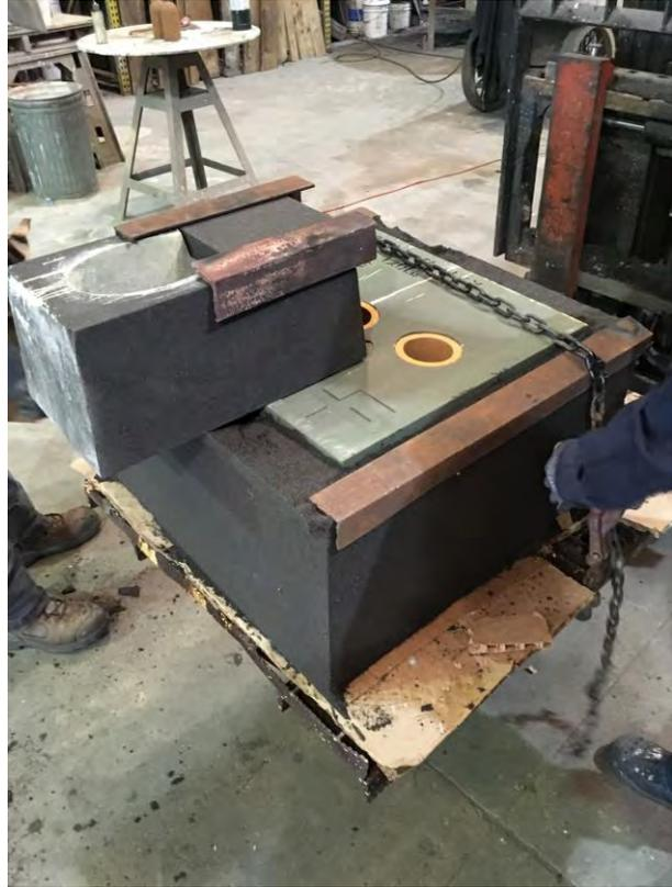
*Figure 7: Assembled mold, ready for pouring.*
