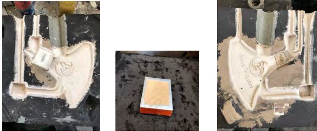
Figure 34: Ceramic sand pattern and core box with refractory paint and exothermic sleeves.
