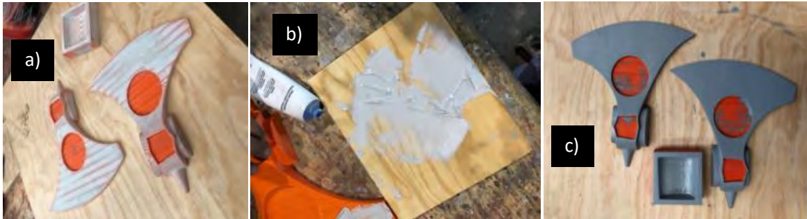
Figure 18: 18a) Pattern with applied paste, 18b) Automotive paste "3M Quick Grip Filler", 18c) Application of protective primer coat.
