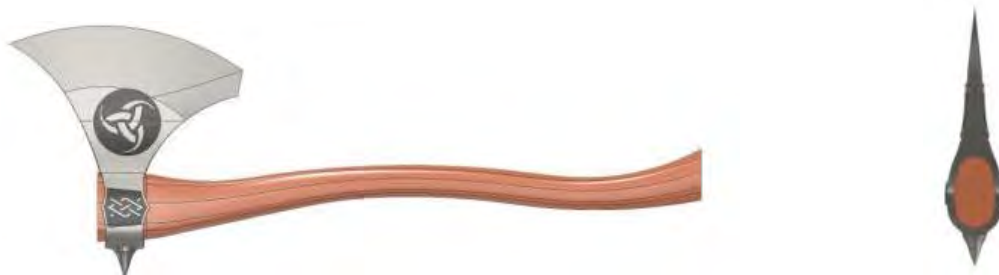
Figure 25: Side and top views for the handle of the axe with a length of 28 in.
