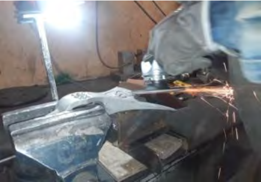
Figure 38: Cutting and sharpening the Viking axe.
