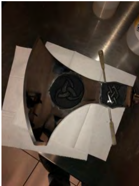
Figure 41: Polishing the axe to have a better surface finish and more striking appearance.
