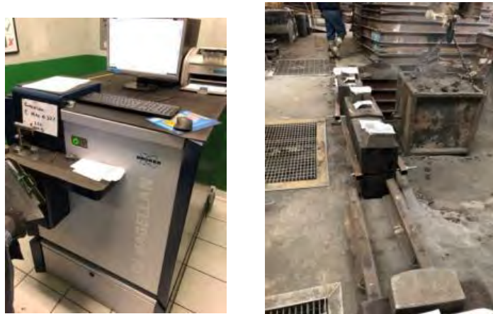
Figure 35: Optical emission spectrometer to analyze samples and molds ready to be poured.
