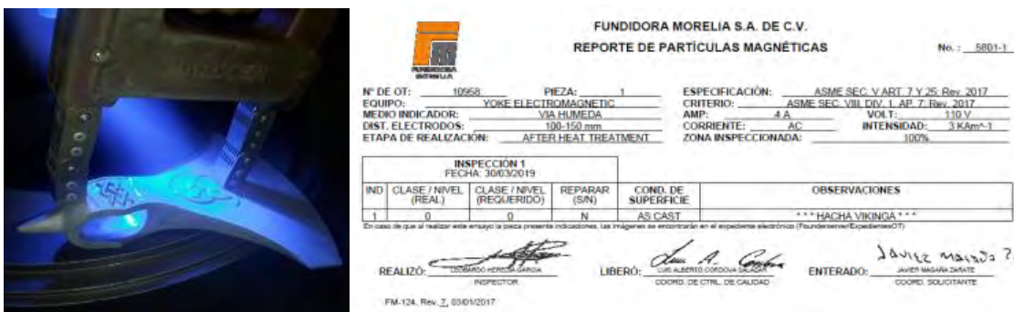
Figure 40: Magnetic particles to visualize defects in the piece and its report.
