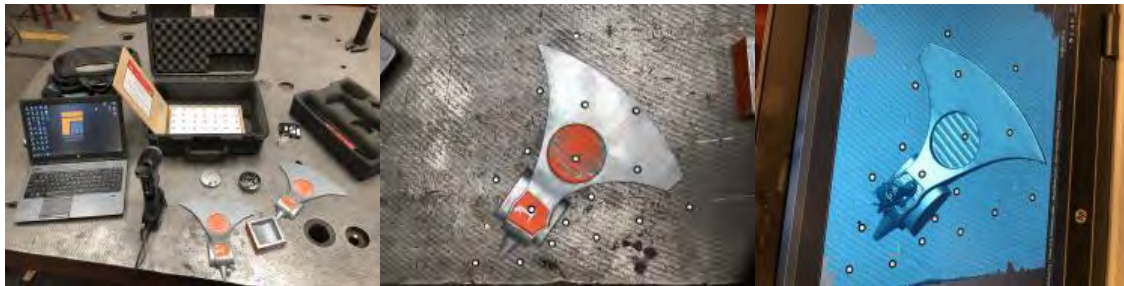
Figure 21: 21a) Handy Scan3D and patterns to scan, 21b) Use of reference labels on a pattern, 21c) Mesh or point cloud generated by the VX Elements software.
