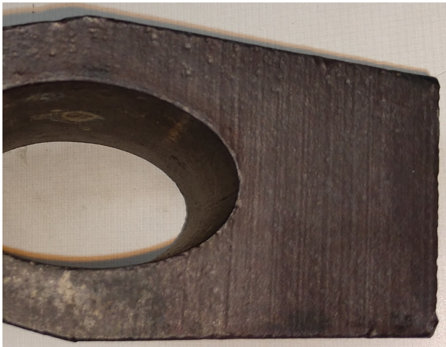
Figure 8: Vertical lines are caused by the 3D printing of the wax pattern
