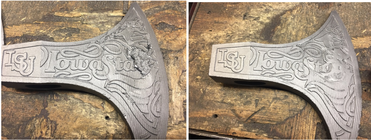
Figure 12: Issue with one side of the axe, before and after grinding
