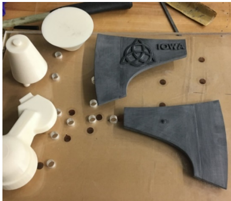
Figure 8. Printed and sanded parts on the plexiglass mounting plate
