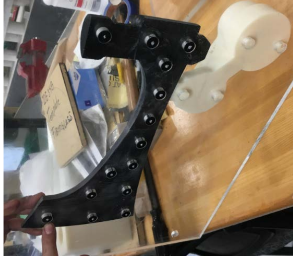
Figure 9. Back part of pattern where bolts would go
