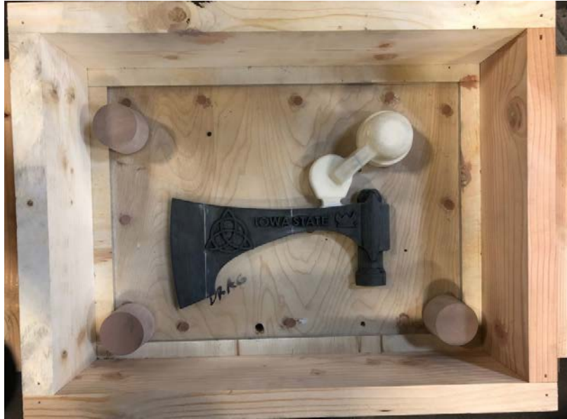
Figure 11. Drag pattern in wooden flask
