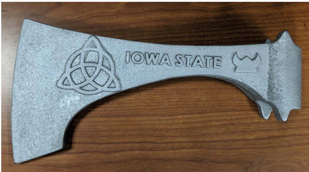
Figure 14. Part after in-gate removed
