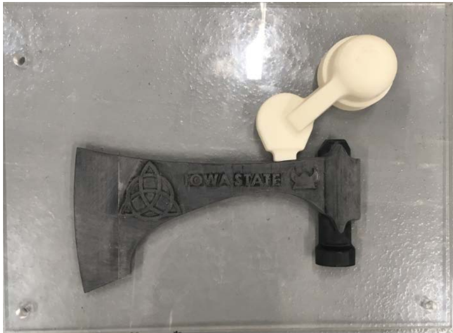
Figure 10. Finished drag side of the pattern
