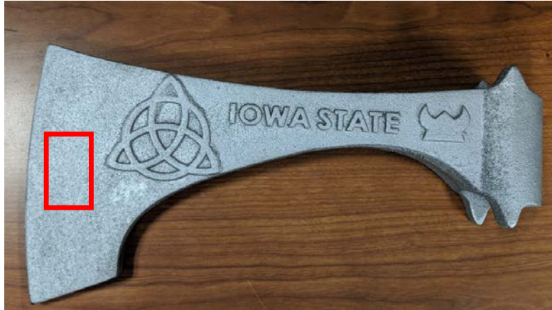
Figure 20. Area evaluated for surface roughness
