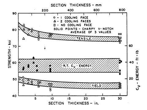
Fig. 15-74 Effect of section size on tensile and impact properties, at the 1/4 T and center locations, of a normalized and tempered turbine blade casting of Ni steel (0.20%C, 2.4%Ni) Conversion: 1 ksi = 6.895 MPa, 1 ft·lb = 1.356 J (1).
