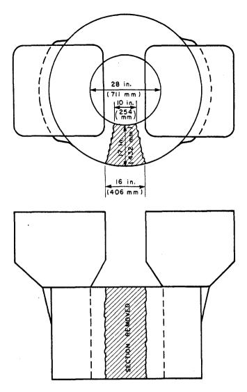
Fig. 15-76 Sketch of cast gear, quenched and tempered cast 8630 steel, showing location of section from which trepanned specimens were removed.
