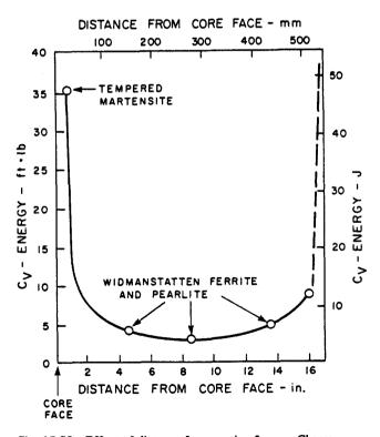
Fig. 15-78 Effect of distance from casting face on Charpy V-notch impact energy at  $0^{\circ}F$  (-18°C) of a gear blank shown in Figure 15-76 (1).
