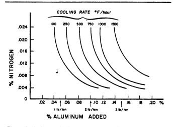
Figure 8. A chart to indicate approximate limits of nitrogen and aluminum that may be tolerated in a base analysis containing 0.30% C, 1.60% Mn, 0.50% Si, 0.50% Cr, and 0.35% Mo without development of intergranular type fracture.
