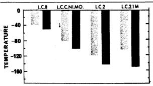
COMPARISON OF N.D.T.T. OF 2" SECTION VS. 5" SECTION
