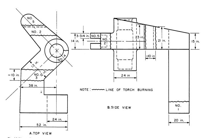
Fig. 15-71 A. Top view of pivot arm with significant dimensions. B. Side view of pivot arm with significant dimensions. Conversion: 1 in. = 25.4 mm.
