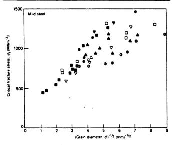
Figure 2. Dependence of local fracture stress of on the grain size of mild steel.
