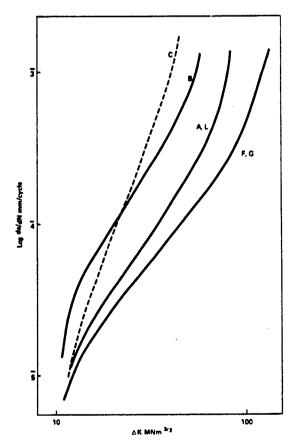
Figure 10. Fatigue crack propagation curves for six steels ( $A=1\frac{1}{2}\%Mn$ ,  $B=\frac{1}{2}\%Cr-\frac{1}{2}\%Mo-\frac{1}{4}\%V$ ,  $C=1\frac{1}{2}\%Mn-\frac{1}{4}\%Ni-\frac{1}{2}\%Cr-Mo$ ,  $F=1\frac{1}{2}\%Mn-Mo$ ,  $G=1\frac{1}{2}\%Ni-Cr-Mo$ , L=0.54%C).
