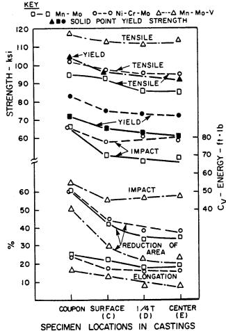
TABLE 15-22 Analyses of Four 5.5 in. (140 mm) Thick Low Alloy Steel Castings (1)
