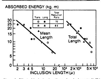
Figure 6. Effect of inclusion length on absorbed energy in the longitudinal and transverse direction.
