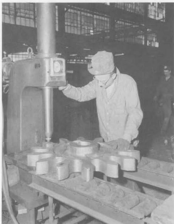
*Brinell testing measures hardness, while below, X-Rays determine internal defects.*
