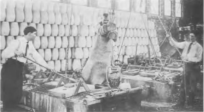
*A Prime Steel Castings Company dramatization of the removal of crucibles from the furnace. Although this photo was taken c. 1905, the principles of crucible operation had not radically changed from the 1860's when steel castings were produced exclusively of crucible steel.*
