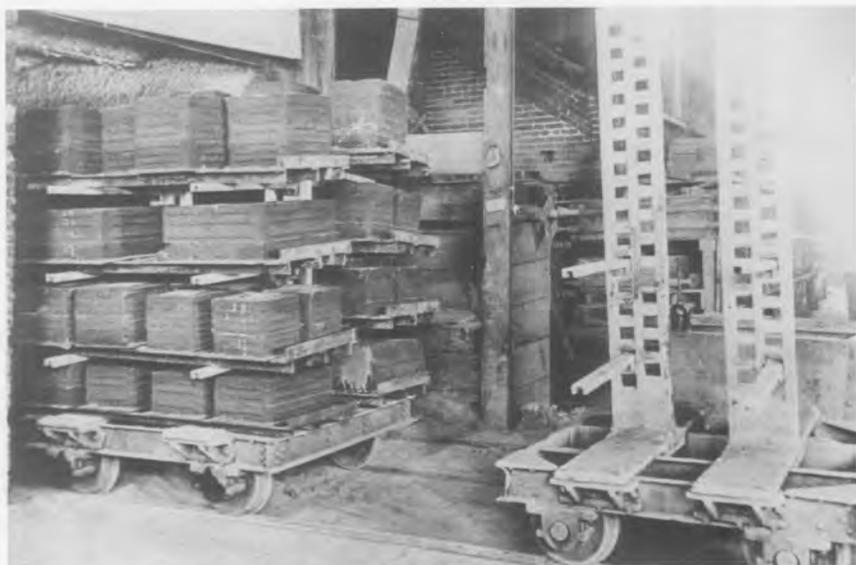
*Drying oven and car with racks to hold dry sand molds.*
