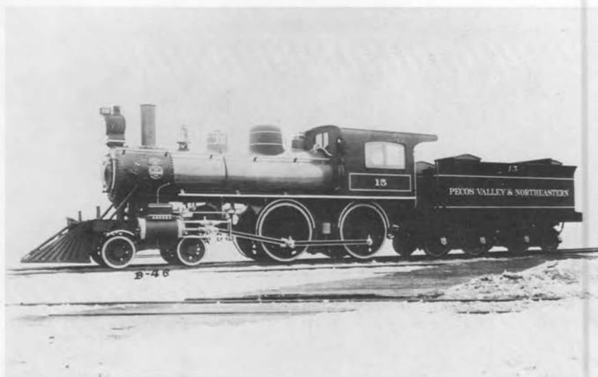
Built during a transition period, 1897-1898, these two locomotives illustrate the link and pin and Janney coupling devices. The Pecos Valley and Northeastern's No. 15 carries a needle-like bar, or link, over the cawcatcher. The Lake Shore and Michigan Southern Railway's No. 316 made use of the Janney coupler which is visible over the catcher.
