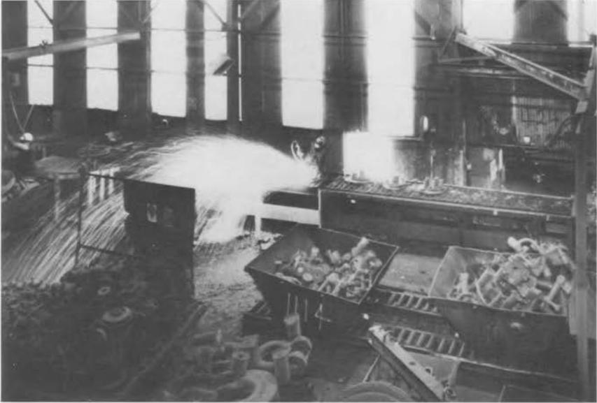
*Hand grinding and welding have cut the amount of time necessary to clean and repair castings.*
