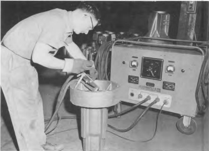
*Magnaflux testing for surface defects.*
