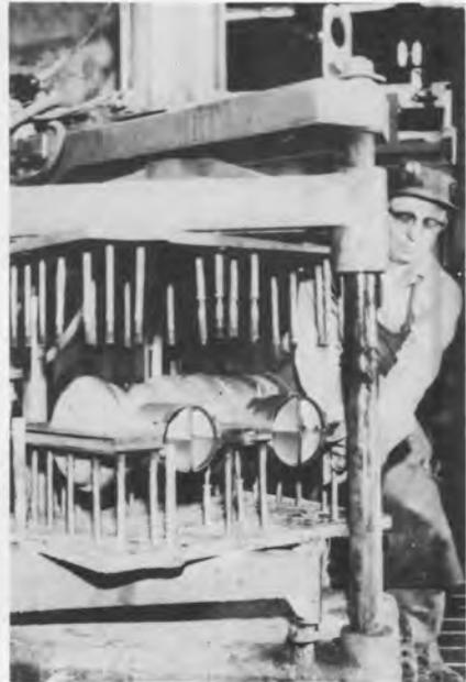
*Shell molding gained increased acceptance during the 1960's as steel foundries competed with the weldments and forging industries. Left, the cope and drag for a valve are removed from a shell molding machine. Right, a shell mold for a track roller is bonded hydraulically.*
