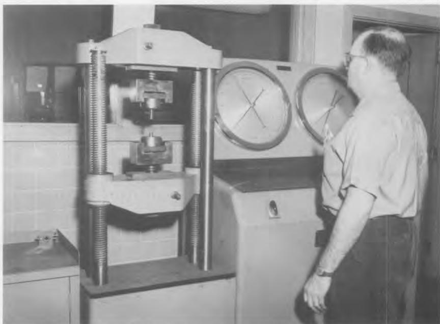
*Physical testing for tensile strength measures elongation and breaking point.*
