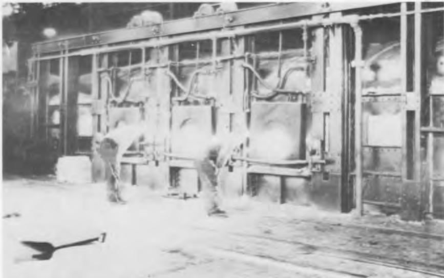
The enormous capacity of the open-hearth accounted for its high percentage of total steel castings production. Above, two melters follow the heat's progress.
