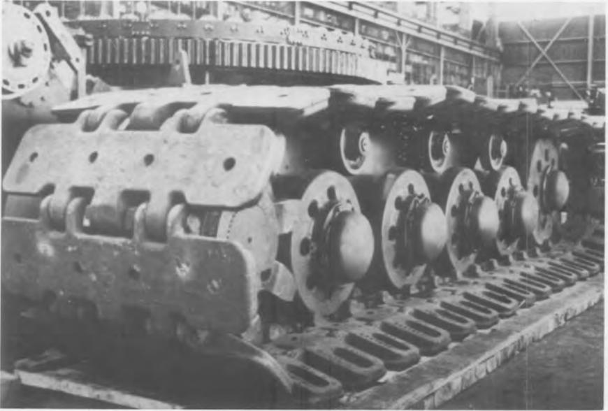
*Modern construction machinery relies heavily upon steel castings. Gears, treads and bucket frames are all cast of steel.*
