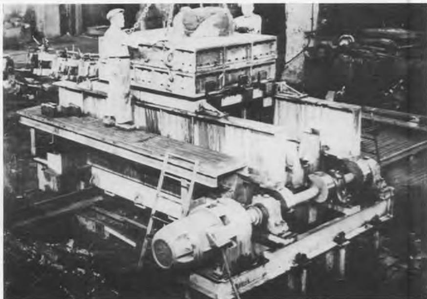
An automatic "shake-up" machine raised and dropped a 20,000 lb. mold 83 times a minute to shake sand from castings.
