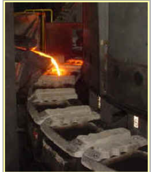
Automated Metal Pouring at Dotson
