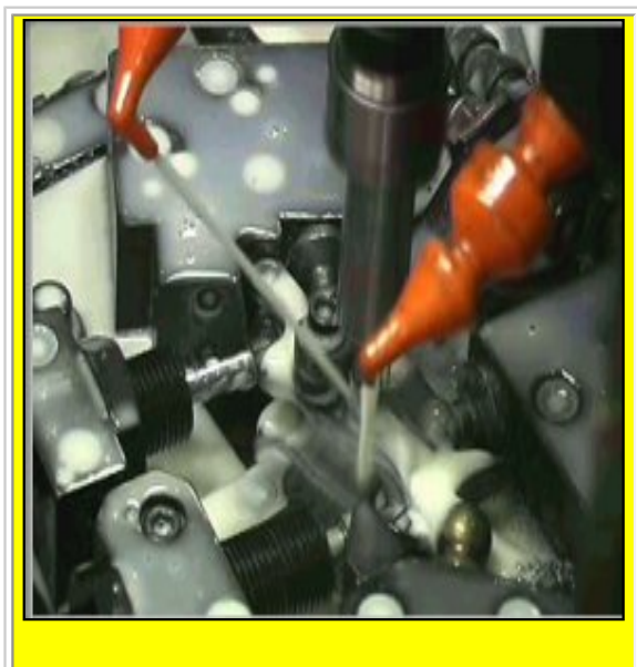
Automated Boring Operation
