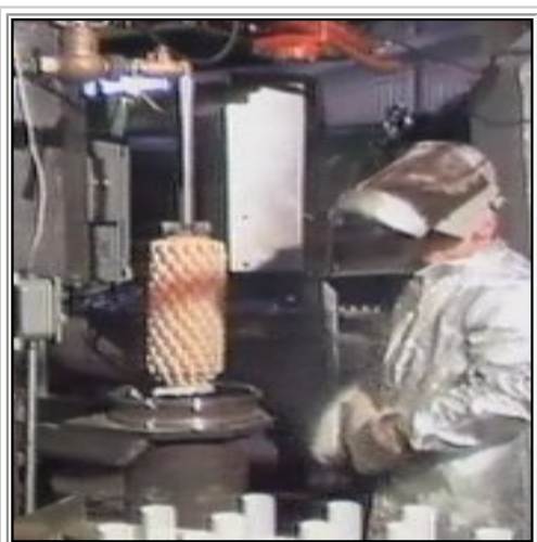
Ceramic Shell Mold
