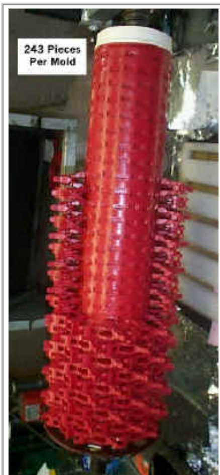
Partial Pattern Assembly before Investment
