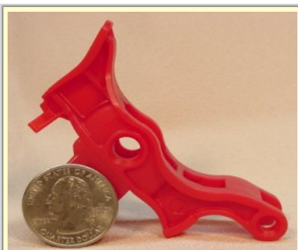
Wax Pattern for Lever Arm
