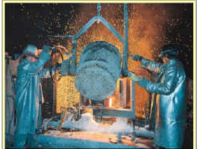
Metal Pouring into a Horizontal Mold
