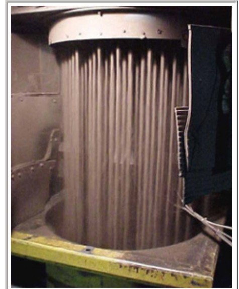
Sand Fill into the Flask (Courtesy of LostFoam.com)
