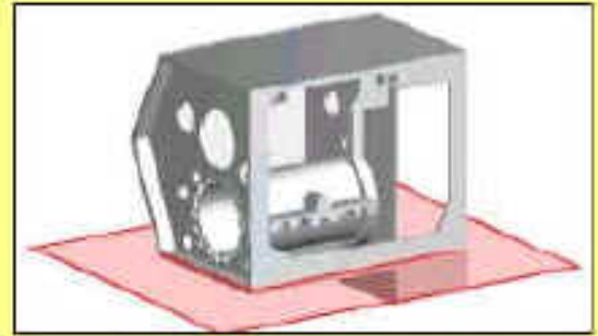
Option A -- Low Parting Line, Base Plate Down
