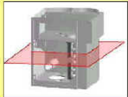
Option C -- Middle Parting Line, Spline Section Down
