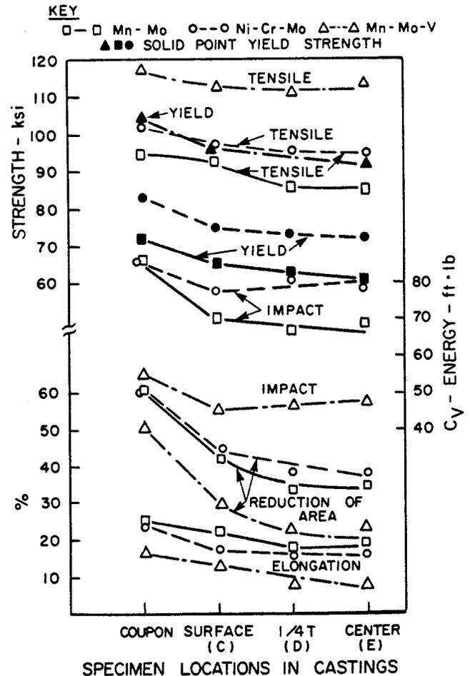
Fig. 15-69 Mechanical properties of specimens cut from various locations of quenched and tempered low alloy steel production castings (Compositions given in Table 15-22) (1). Conversion: 1 ksi = 6.895 MPa, 1 ft·lb = 1.356 J.
