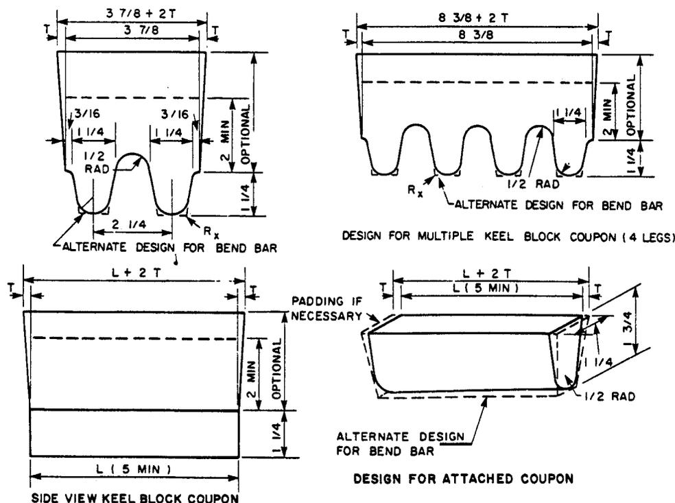
Fig. 15-67 Keel block coupon (ASTM A370—mechanical testing of steel products). Conversion: 1 in. = 25.4 mm.
