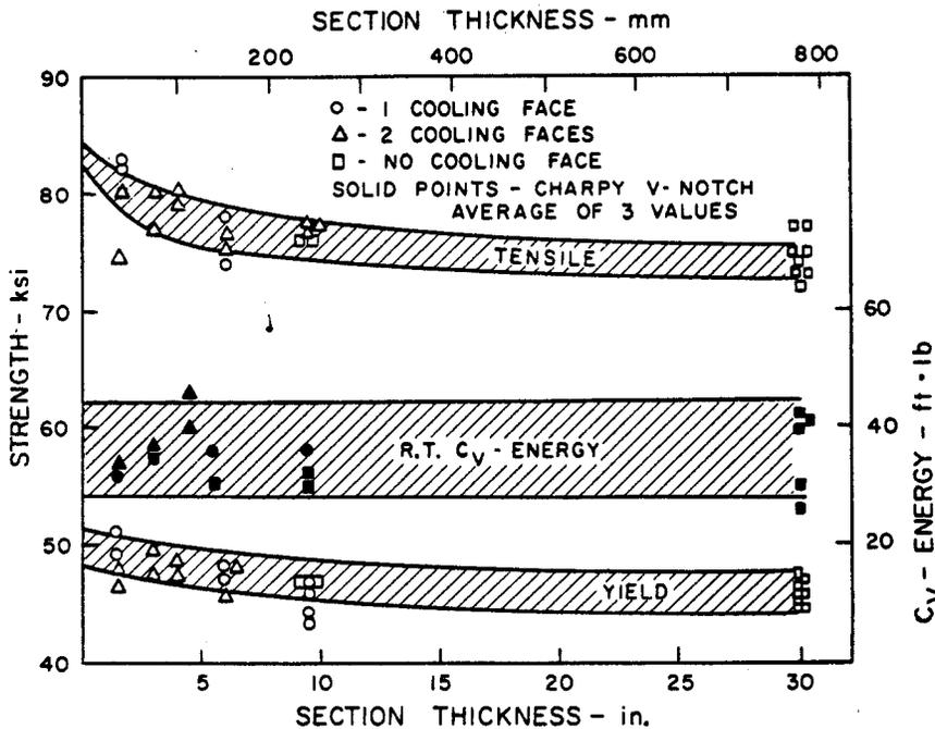
Fig. 15-74 Effect of section size on tensile and impact properties, at the 1/4 T and center locations, of a normalized and tempered turbine blade casting of Ni steel (0.20%C, 2.4%Ni) Conversion: 1 ksi = 6.895 MPa, 1 ft·lb = 1.356 J (1).
