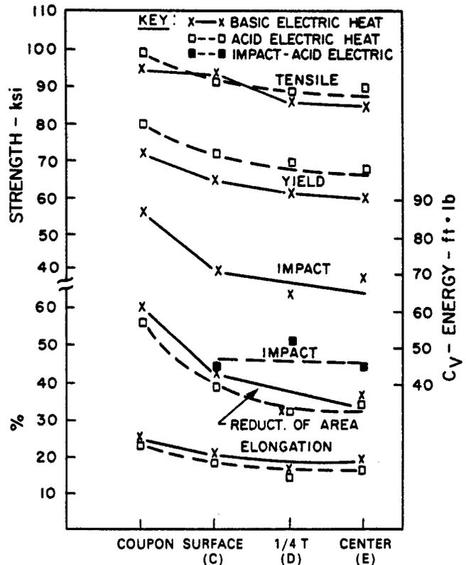
FIG. 15-68 Mechanical properties of specimens cut from various locations of two quenched and tempered Mn-Mo production castings (Composition in Table 15-22) (1). Conversion: 1 ksi = 6.895 MPa, 1 ft·lb = 1.356 J.
