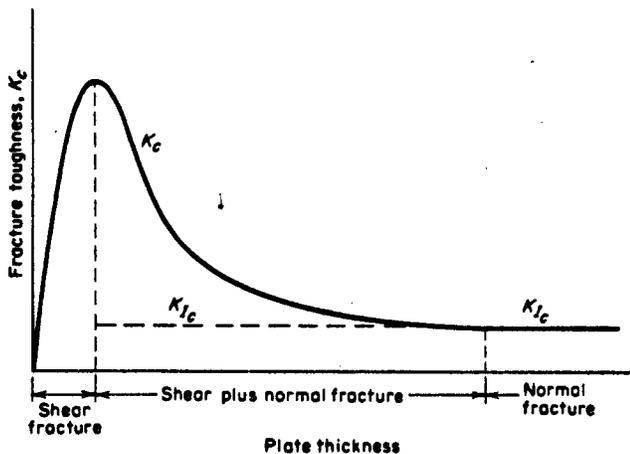
Figure 9. Schematic variation of the fracture toughness as a function of the plate thickness.
