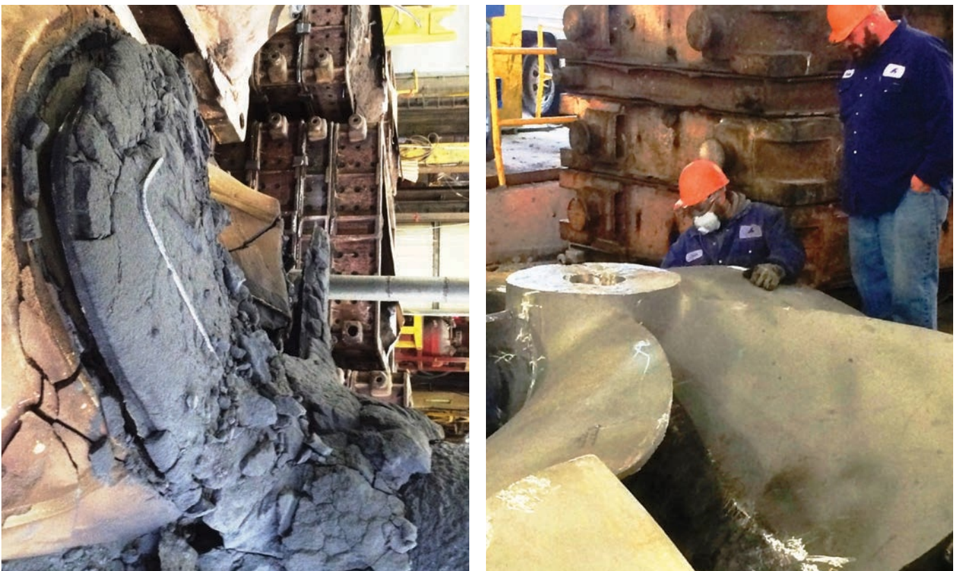
Fig. 1 — A propeller is cast in sand in a foundry (left). On the right is the propeller casting with the sand removed.
