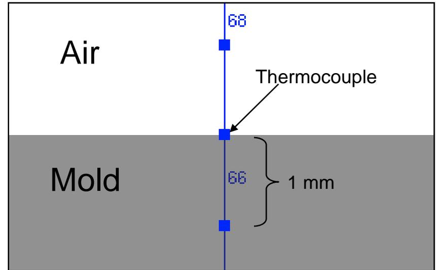
Thermocouples placed at the surface of the mold.
