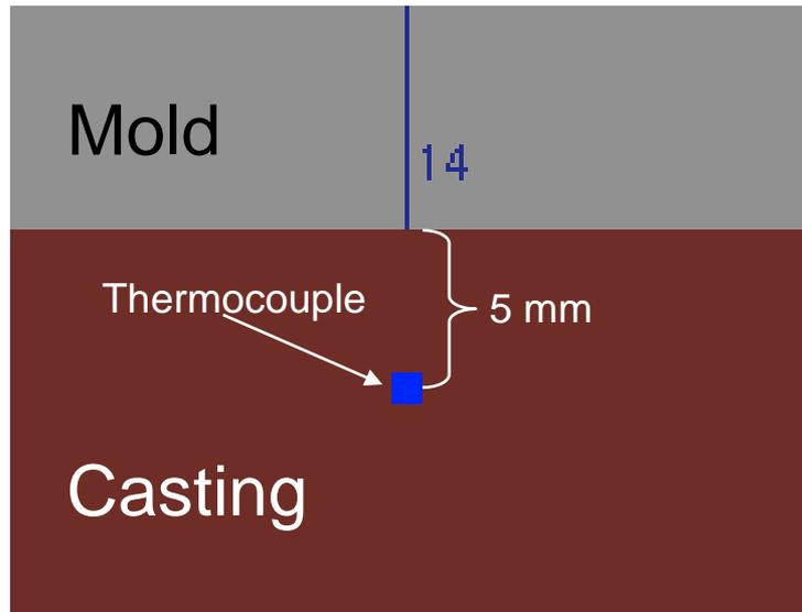
Thermocouple placed 5 mm into steel casting.
