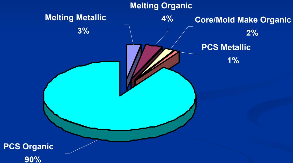
For typical large greensand cored foundry with wet scrubber.
