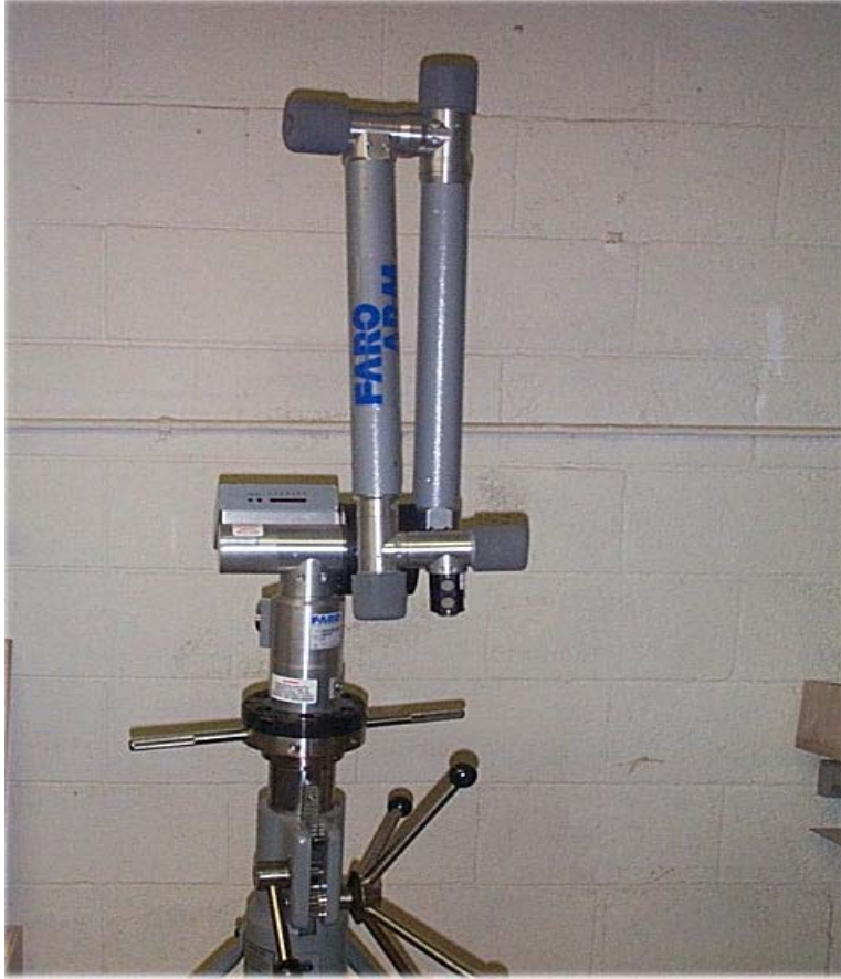
8' FaroArm, Silver Series S-08-02-US-IN CAM2 Measure System ACME-NC-US-POR Serial #S08029901487 Model S08-02
