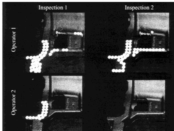
**Fig. 10b. Pictures of defects marked on the same specified location on a second casting four different times. Same method used; two inspectors each inspected the same part twice.**
