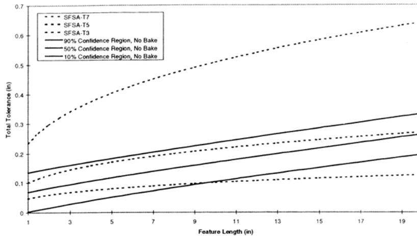
**Fig. 7. Long series production – No bake dimensional capabilities compared to SFSA T-Grades**
