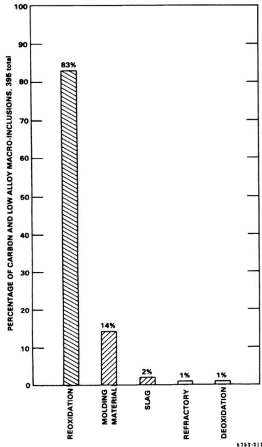
**Fig. 1. Distribution of macroinclusion sources in carbon and low alloy steel castings**
