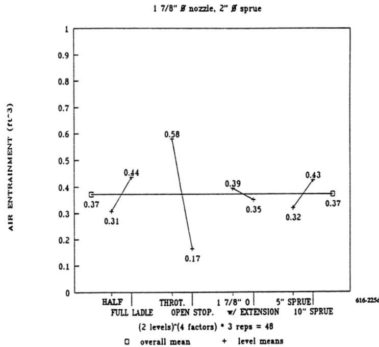
**Fig. 3. Mean effects diagram for bottom pouring factors in water modeling series 1**
