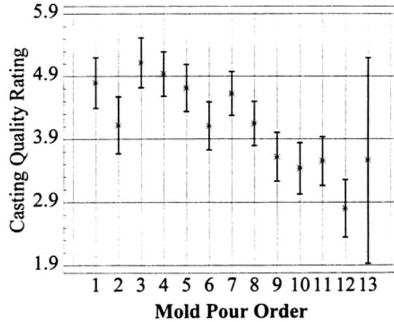
**Fig. 5. Effect of head height on casting quality at basic foundry**
