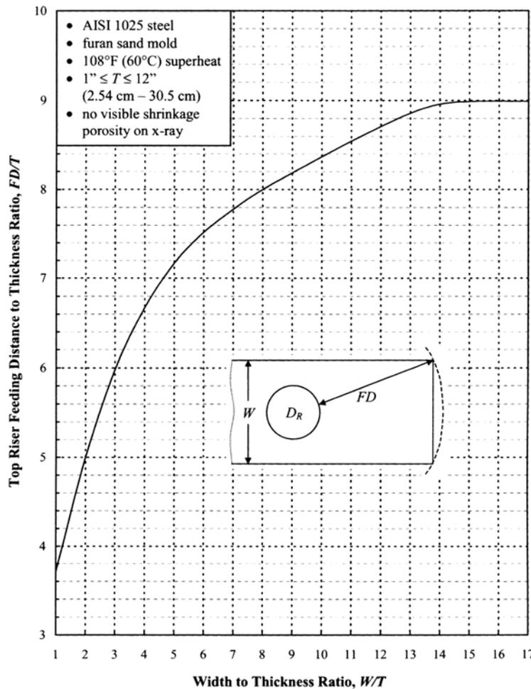
**Fig. 8. Feeding distance (FD) as a function of width and thickness for top-risered sections cast with plain carbon steel**
