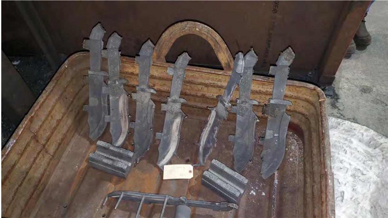
**Figure 8. Raw castings after degating are shown.**
