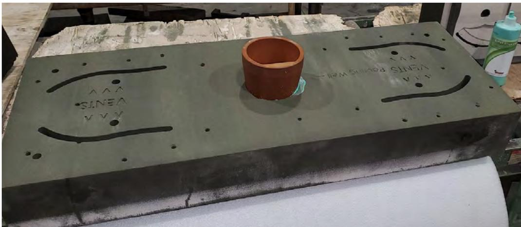
**Figure 5. Modifications to the mold such as larger pour cup and vents can be seen above.**
