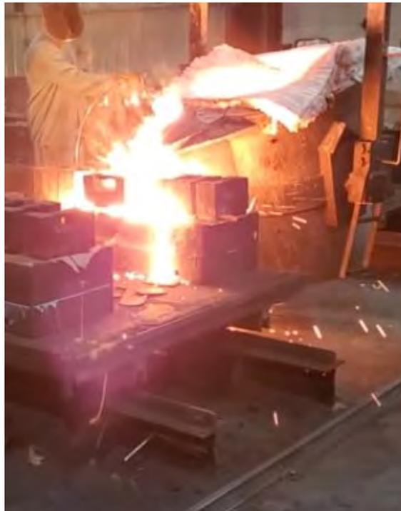
**Figure 7. A bowie knife mold being poured at Omaha Steel is shown.**
