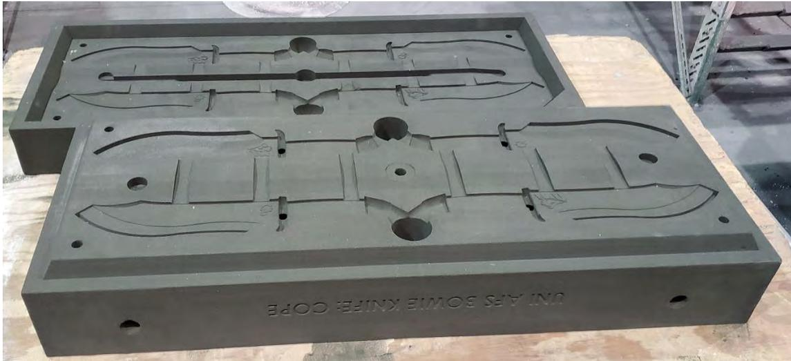
**Figure 4. Above is a picture of the 3d printed mold**
