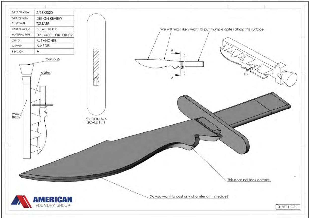
Figure 4: Initial Bowie Knife model (With Guard and Risers)
