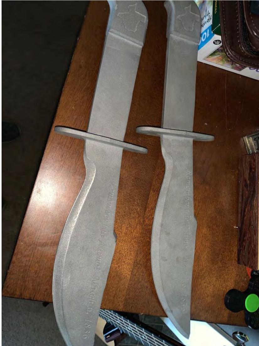
*Figure 8: Raw Bowie Knife Castings received from AFG*
