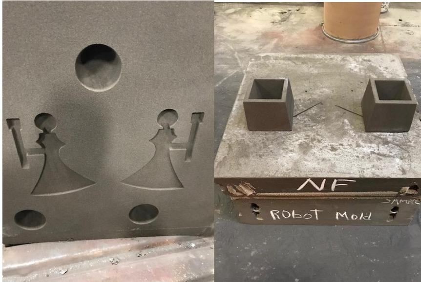
**Figure 1:** The drag side of the mold on the left, and the closed and completed mold on the right.
