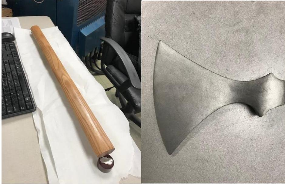
**Figure 4:** The handle after finishing with linseed oil, and the axe head after the final stainless steel shot blast.
