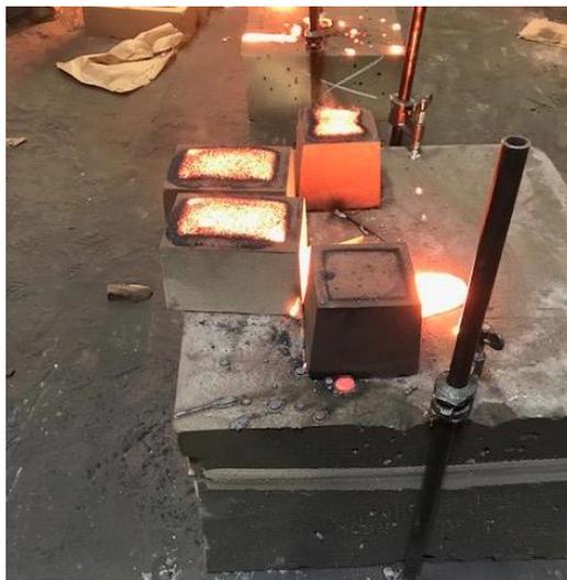
**Figure 2:** The axe heads and keel blocks immediately after pouring, with the addition of hot top.
