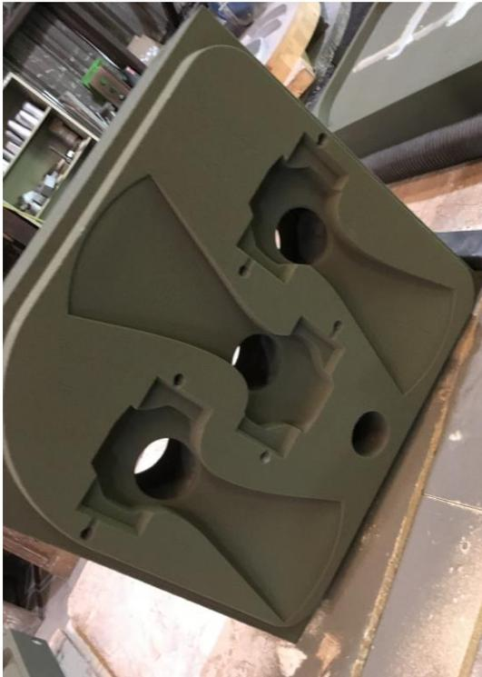
*Figure 6: 3D printed mold for casting. With holes for risers visible.*
