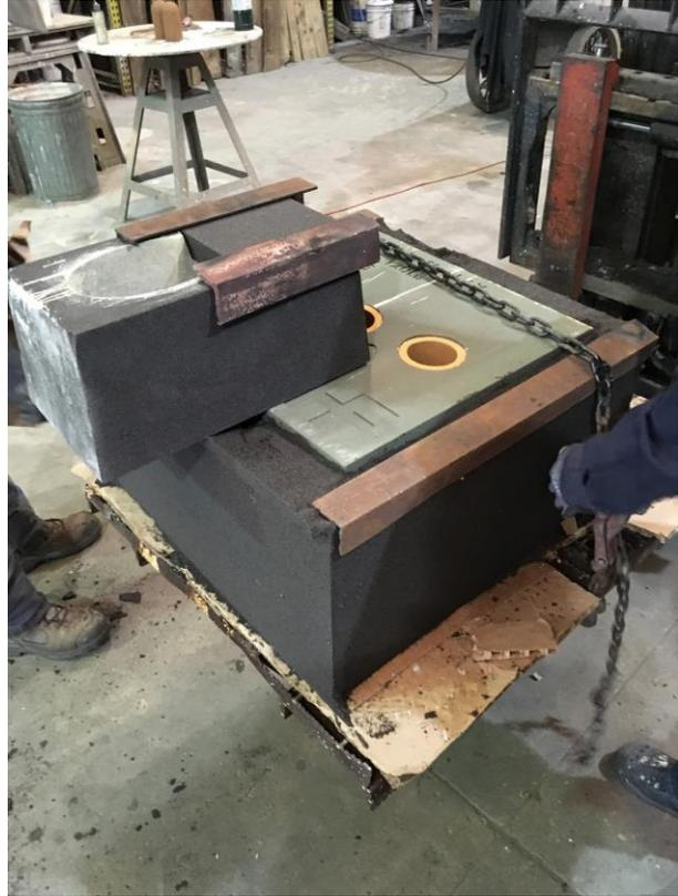
*Figure 7: Assembled mold, ready for pouring.*
