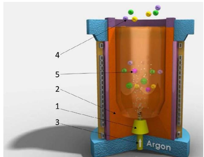
Figure 1. Porous Plug and Injection of Argon Gas Through the Bottom in Induction Furnaces configuration.
