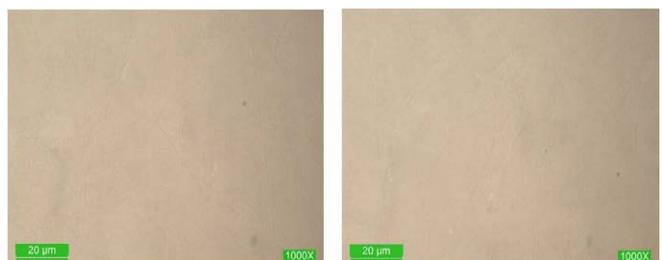
Figure 19 b). heat number 20K8E without etching at 1000X CF8C material.
