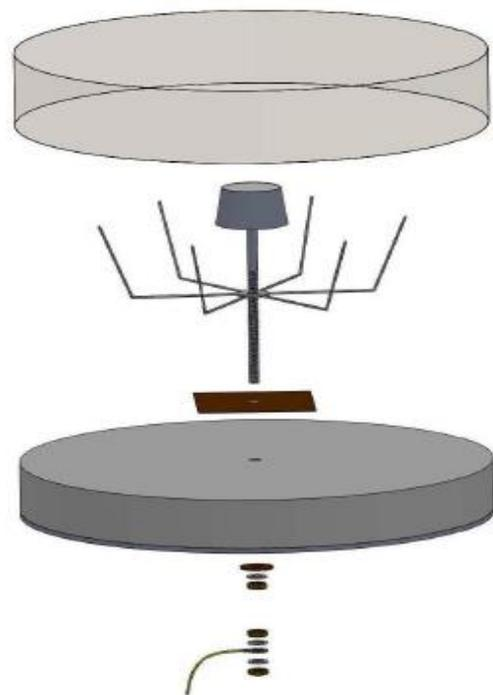
Figure 3. Typical diffuser installed in the center of the IF base (exploded view)
