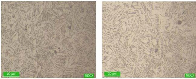
Figure 13 a). heat number 19S37H with etching at 1000X LCB/LCC material – Nital 5%.
