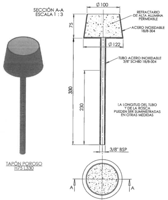
Figure 5. Porous plug components. Scale 1:3.
