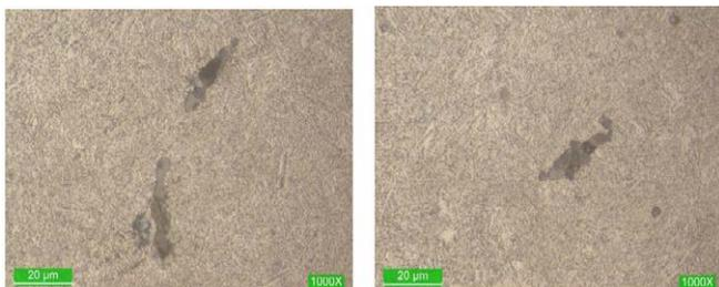
Figure 15 a). heat number 19T14F with etching at 1000X 86xx material – Nital 5%.
