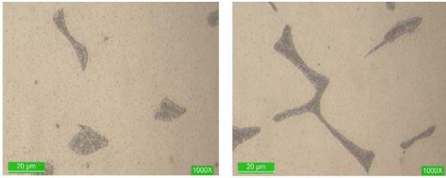
Figure 20 a). heat number 19J87F with etching at 1000X CF8C material.
