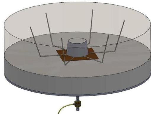
Figure 2. Typical diffuser installed in the center of the IF base (assembly)
