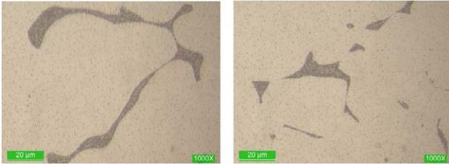
Figure 20 b). heat number 20K8E with etching at 1000X CF8C material.
