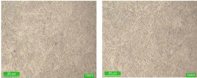
Figure 13 b). heat number 20N16H with etching at 1000X LCB/LCC material – Nital 5%.
