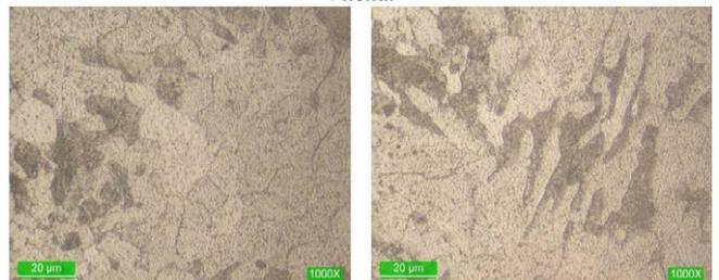
Figure 17 b). heat number 20K37H with etching at 1000X WC6 material – Vilella.
