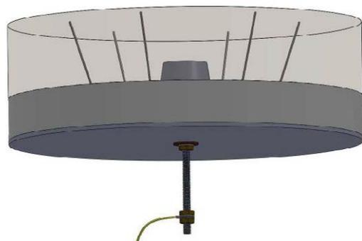
Figure 4. Typical diffuser installed in the center of the IF base (bottom)
