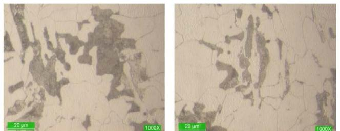
Figure 11 b). heat number 20N18H with etching at 1000X WCB/WCC material – Nital 5%.
