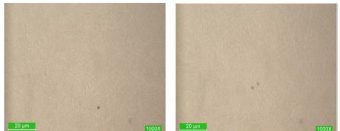
Figure 12 b). heat number 20N16H without etching at 1000X LCB/LCC material.
