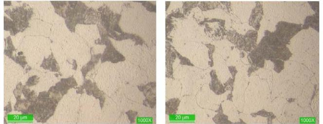
Figure 11 a). heat number 19K37H with etching at 1000X WCB/WCC material – Nital 5%.
