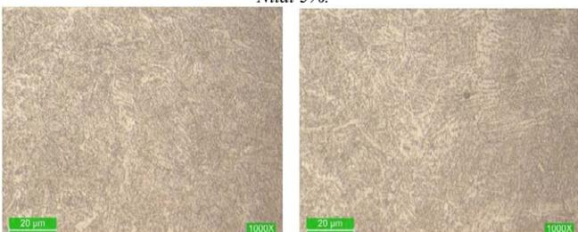
Figure 15 b). heat number 20K42H with etching at 1000X 86xx material – Nital 5%.
