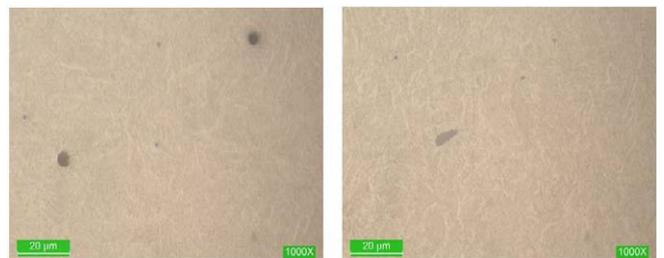
Figure 12 a). heat number 19S37H without etching at 1000X LCB/LCC material.
