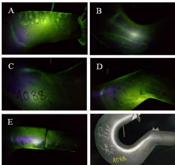
Figure 11. heat code: A088, Photos of castings after final MT. No cracks found.
