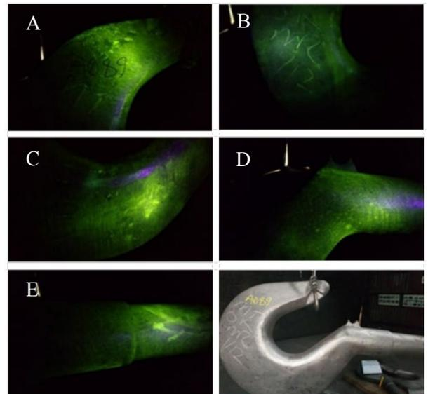
Figure 12. heat code: A089, Photos of castings after final MT. No cracks found.
