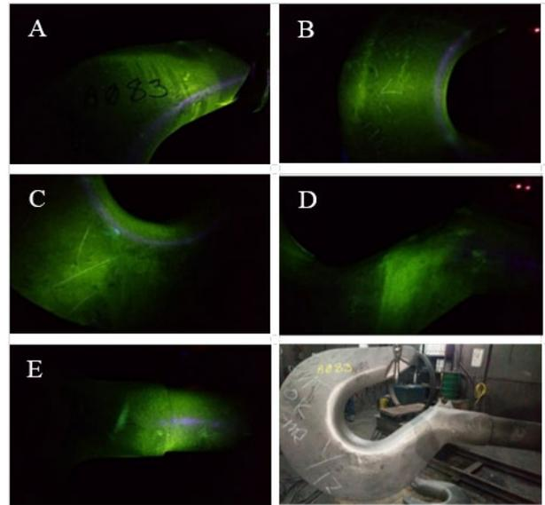
Figure 6. heat code: A083, Photos of castings after final MT. No cracks were found.
