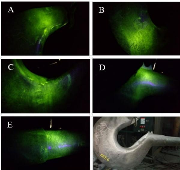
Figure 9. heat code: A086, Photos of castings after final MT. No cracks found.
