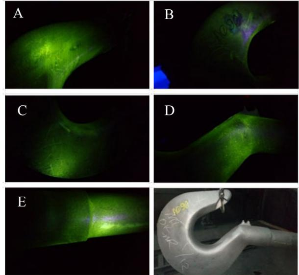
Figure 13. heat code: A090, Photos of castings after final MT. No cracks found.
