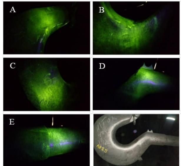
Figure 8. heat code: A085, Photos of castings after final MT. No cracks found.
