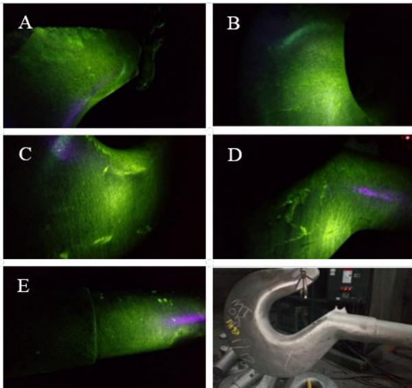
Figure 10. heat code: A087, Photos of castings after final MT. No cracks found
