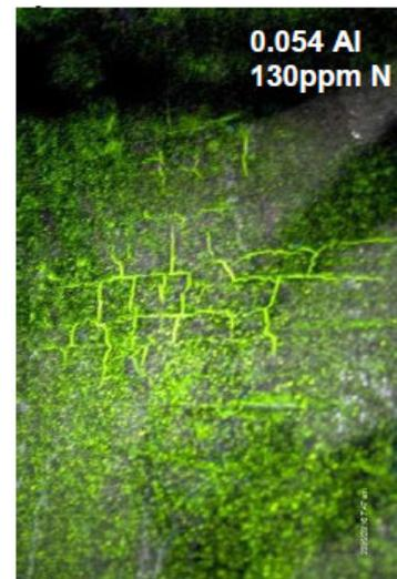
Figure 1. Typical appearance of aluminum nitrides.
