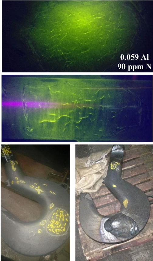
Figure 2. Example AlN cracking found in hook castings.
