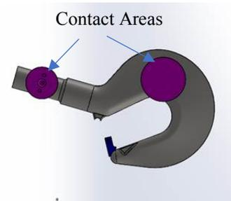
Figure 3. Contact areas. Part Description: 130 Ton Hook, Gross Weight 580 kg.
