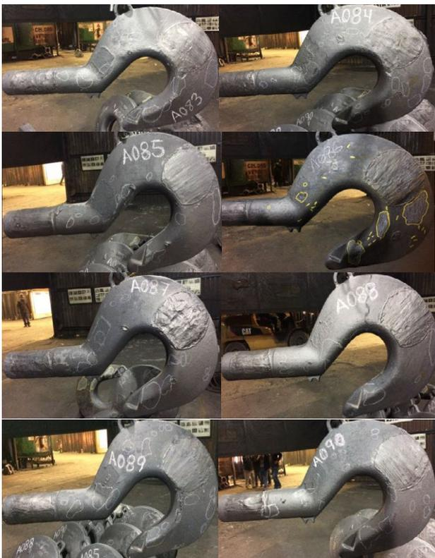
Figure 5. Photos of castings after visual and MT inspections, after Q&T. heat codes: A083, A084, A085, A086, A087, A088, A089, A090.
