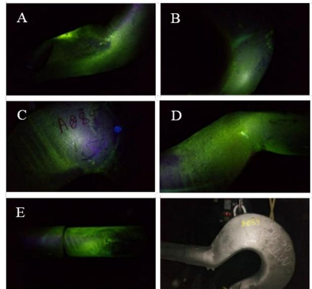
Figure 7. heat code: A084, Photos of castings after final MT. No cracks found.
