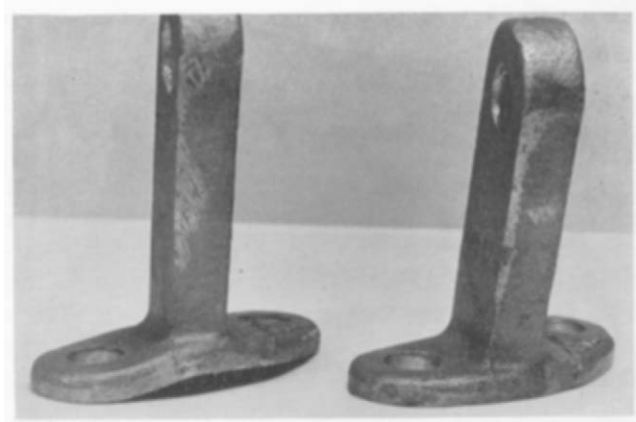
Figure 22—Result of 25,000-pound load on Fulcrum Bracket.
