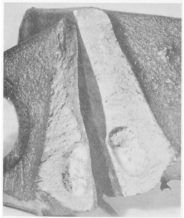
Figure 13—Severe gas porosity in base of Fulcrum Bracket.
