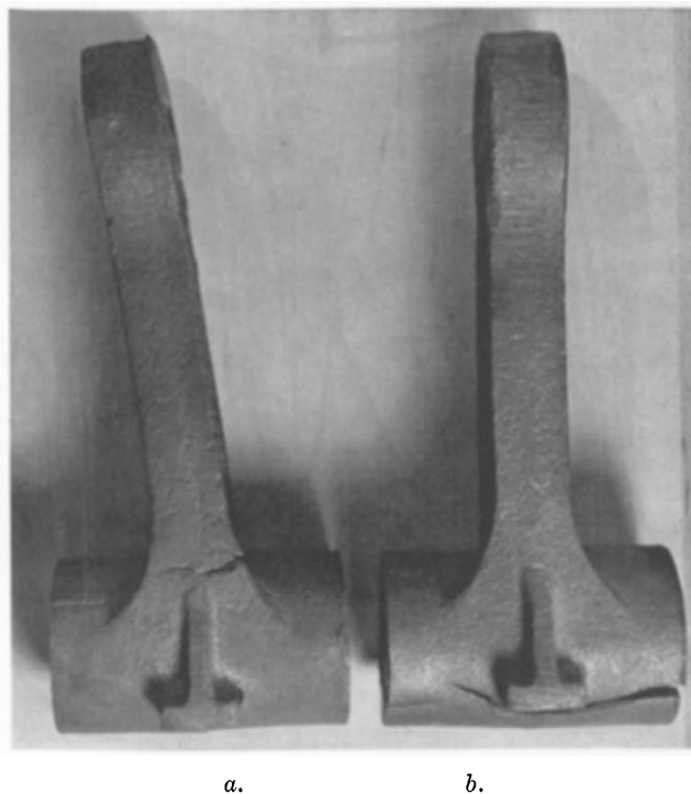
a. b. Figure 39—Types of fatigue failure found in the Lever castings (a) One of two castings loaded at 7700-pound maximum load after 17,300 cycles. (b) Typical failure exhibited by all other Lever castings at lower maximum loads and larger number of cycles.
