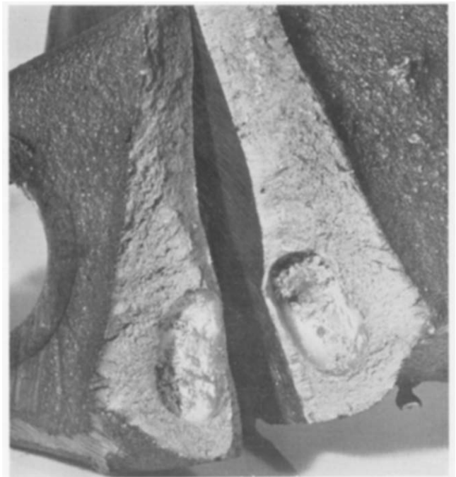
SEVERE GAS POROSITY IN BASE OF FULCRUM BRACKET
