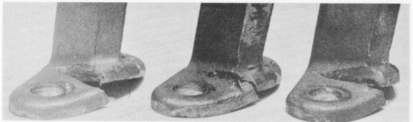
Figure 20—Location of fatigue failures in Fulcrum Bracket.
