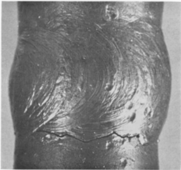
Figure 16—Illustrates Fatigue Crack and Fractured Surface of Sound Weld Torsion Fatigue Cast Steel Specimen.
