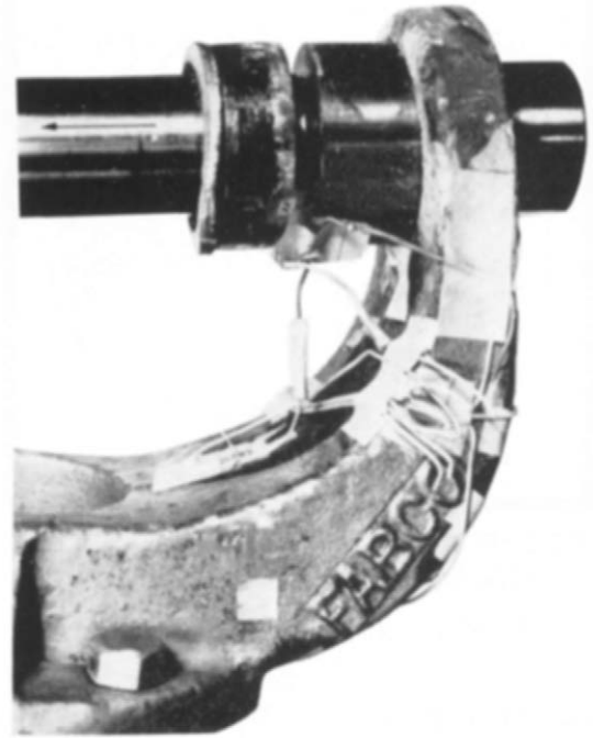
TESTED CASTING SHOWING FAILURE
