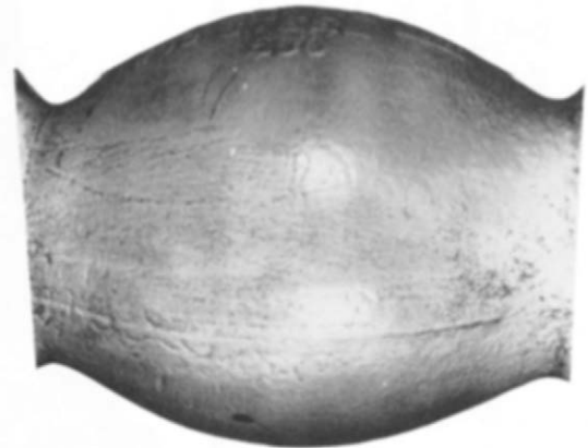
TESTED CASTING SHOWING STRESS COAT PATTERN
